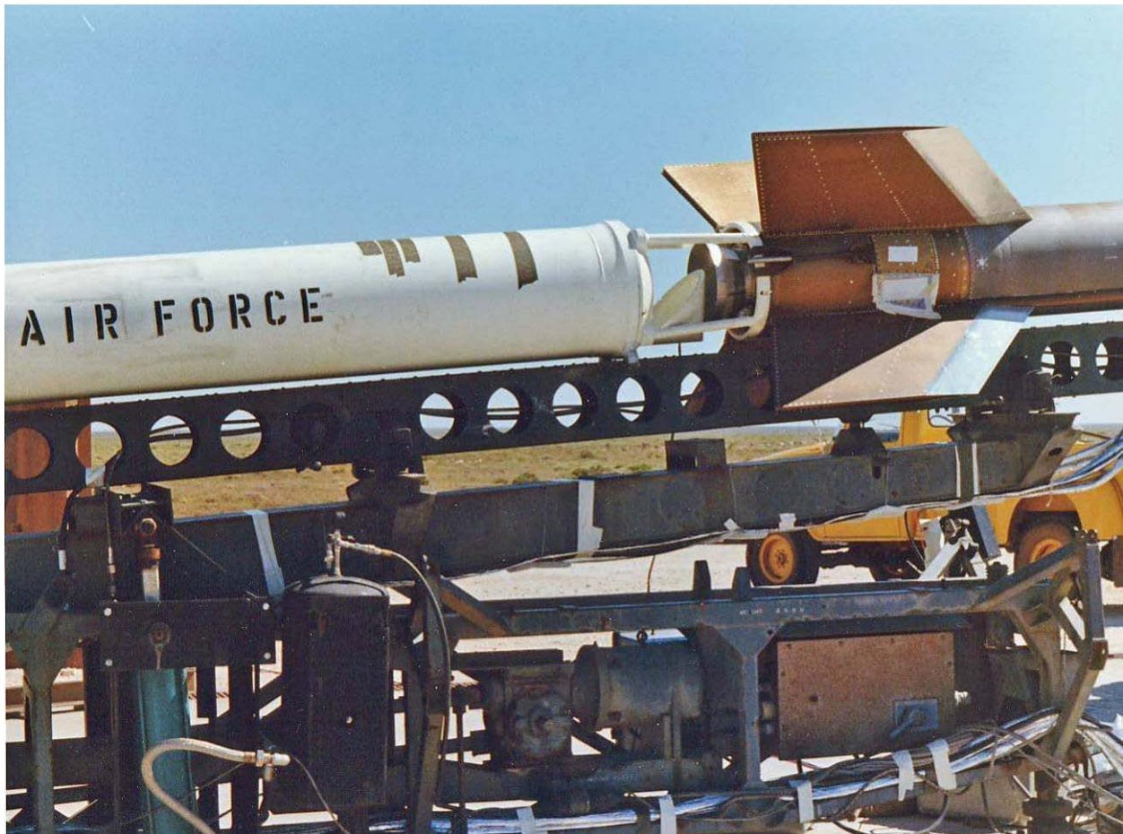
Figure 22. The Nike booster on the launch rail. The rail shoe is the attachment below and at the top of the white “Air Force” booster, which fits over a rail flange and holds the booster to the rail. During launch the shoe slides up the rail flange, which guides the motion of the vehicle.
