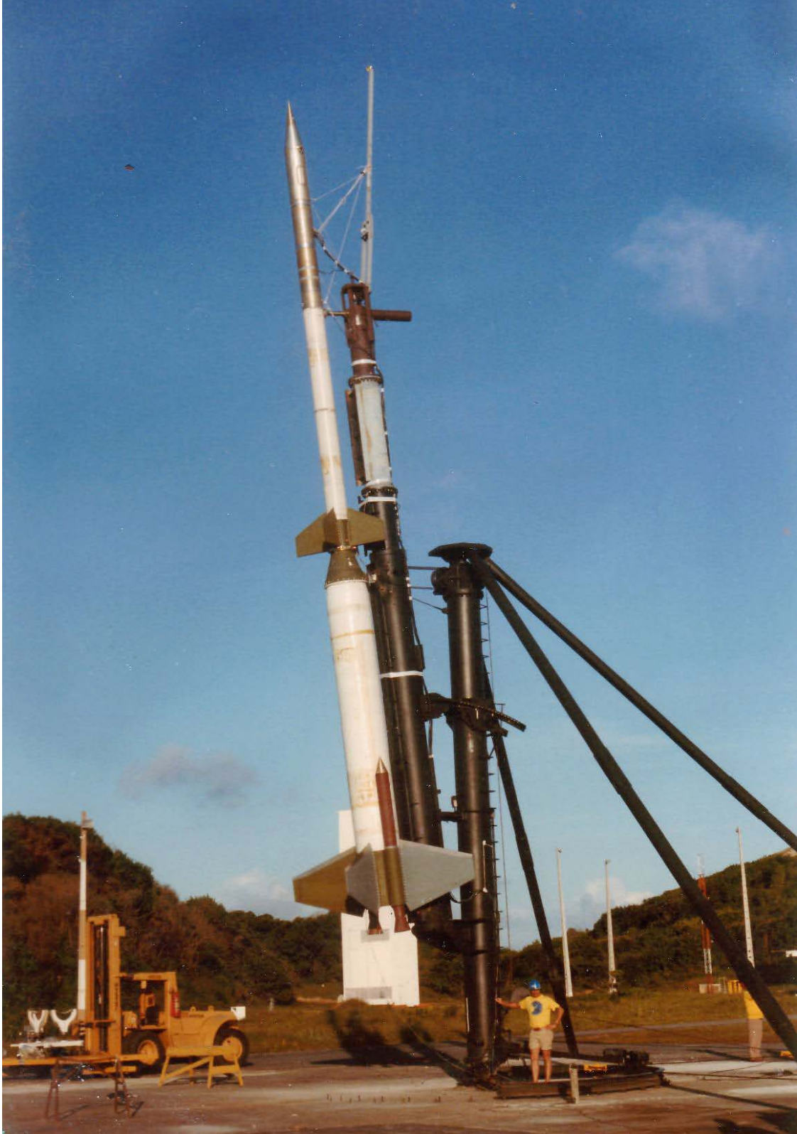
Figure 68. The BEAM experiment mated to the Castor-Lance rocket, which is mounted on the launch rail at the rocket range near Natal, Brazil. Dave Akerstrom is leaning against the launcher and scales the size of the assembly in this photograph.
