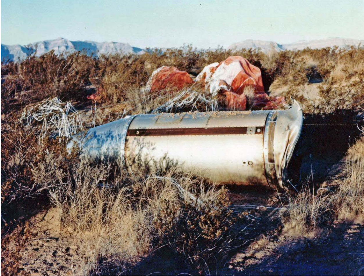
Figure 43. The not so soft SPICE I recovery. The payload impact was much harder than anticipated with the standard recovery pack used on this mission. Despite the appearance, the internal damage was limited.
