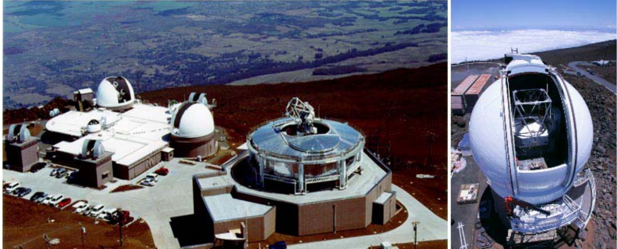
Figure 8. The Air Force Maui Optical Station (AMOS) atop Mt. Haleakala, Hawaii at an altitude of 3054 meters. In the image on the left, the 3.67 m Advanced Electro-Optical System (AEOS) at the right is the largest optical telescope designed to track satellites (Mayo, 1999) and is currently used for most of the infrared imaging, photometry and spectroscopy (Witte, Landee and Musial, 1999). The telescope housing collapses as shown to avoid the problems associated with rotating a massive dome at the 15°/sec needed to track satellites. Dual 1.2 m telescopes in the dome on the back of the building roof at left are mounted on opposite sides of a single polar axis and are aligned to a common declination so that they can track and observe the same object; the larger dome houses a 1.6 m telescope (Lambert, 1999). Both these facilities have been used for infrared observations (Chapman, 1981). The three grey domes enclose a 0.4 m and two 1 m Ground-based Electro-Optical Deep Space Surveillance system (GEODSS) telescopes. The newest facility, the 1.8 m PanSTARRS-1 telescope, shown on the right is outside the left hand image in front of the AEOS. Information and image are taken from http://www.maui.afmc.af.mil/gallery.html .
