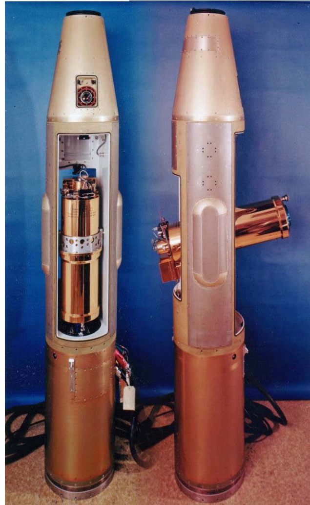
Figure 17. A schematic of the HI STAR payload is at left and the payload section from the telemetry antenna to the nose cone separation line is shown above with the HI STAR sensor stowed and deployed (with cap on).
