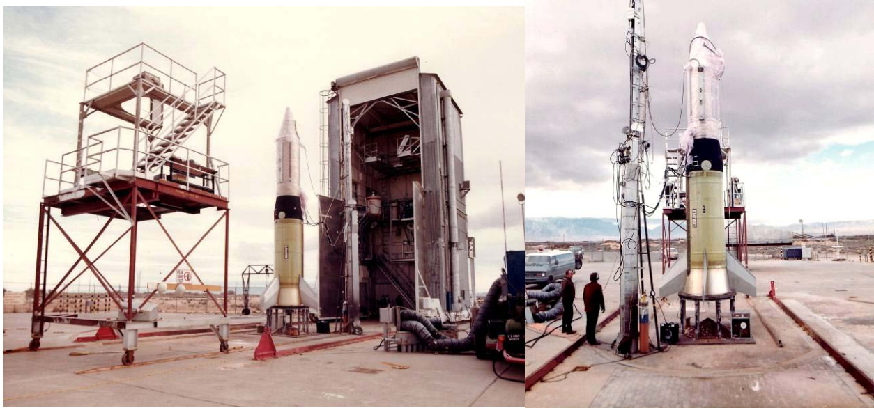
Figure 51. A view of the payload on the rocket with the gantry and preparation building rolled back. The assembled experiment seen from the preparation building is on the right during t-3 hour check.
