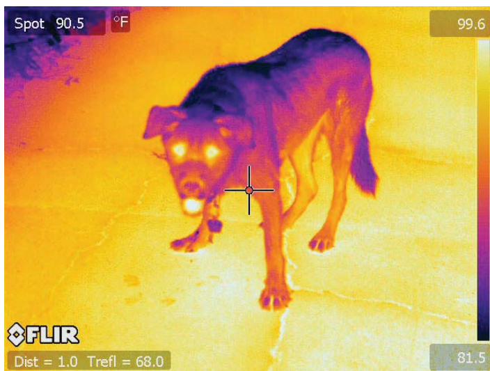
An infrared image of a dog, with warmest areas appearing the brightest.
